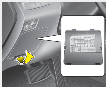
Inner panel fuse panel
